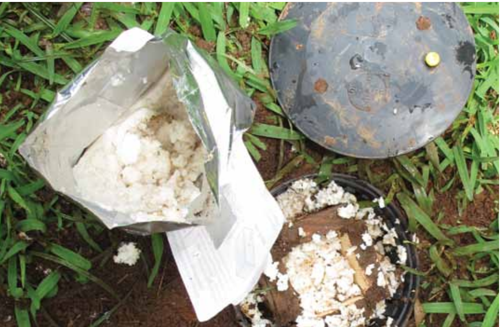
Holes 'mudded up' confirming termites are present in the In-Ground Station.
